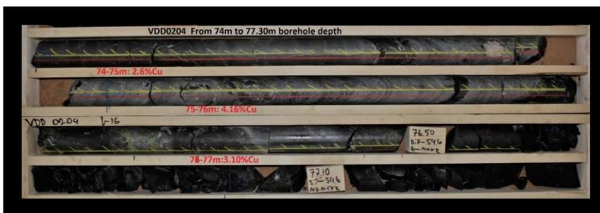
**Drilling highlights of the above holes were: Viscaria A-zone drillings: VDD0203 returns 20m @1.27% Cu, including 5m @2.99% Cu. VDD0204 returns 18m @1.18% Cu, including 3m @3.28% Cu. Significant potential for cobalt and gold.**
